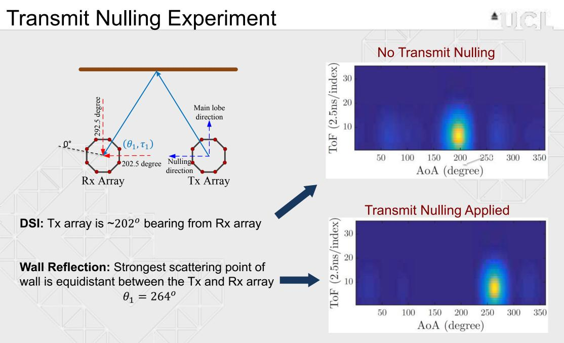
\*ToF difference between DSI and wall reflection path is  $2.5 \text{ ns} \sim 75 \text{ cm}$
