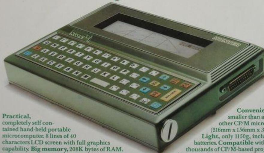
**Practical,** completely self contained hand-held portable microcomputer. 8 lines of 40 characters LCD screen with full graphics capability. **Big memory,** 208K bytes of RAM. 48K operating system ROM. Huge memory capacity for disk emulation. **Rugged** heavy duty metal case and sealed keyboard for use anywhere. **Dependable** fail-safe battery system, choice of rechargeable or alkaline cells.
