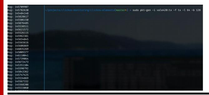
Output when monitoring CPU cycles of an 'fromdevice element' every 0.1seconds
